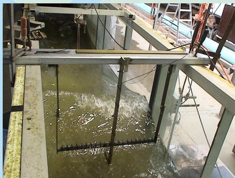
Ongoing increases in ship size have dictated a demand for deeper water berths and therefore longer jetties. In many locations, construction of protective breakwaters for these jetties is not economically viable. Increasingly therefore, jetties are constructed without protection and have to be able to cope with wave forces acting directly upon them. The frequent use of pile supported coastal structures makes the interaction of waves and piles of
